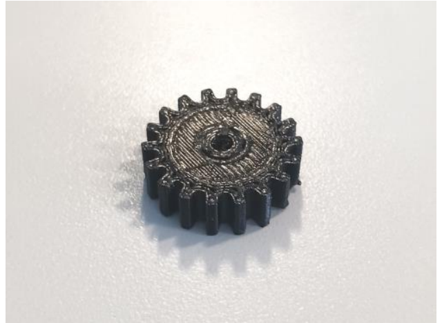
AR4_SG1_gear (3D print – PETG 50% infill)
